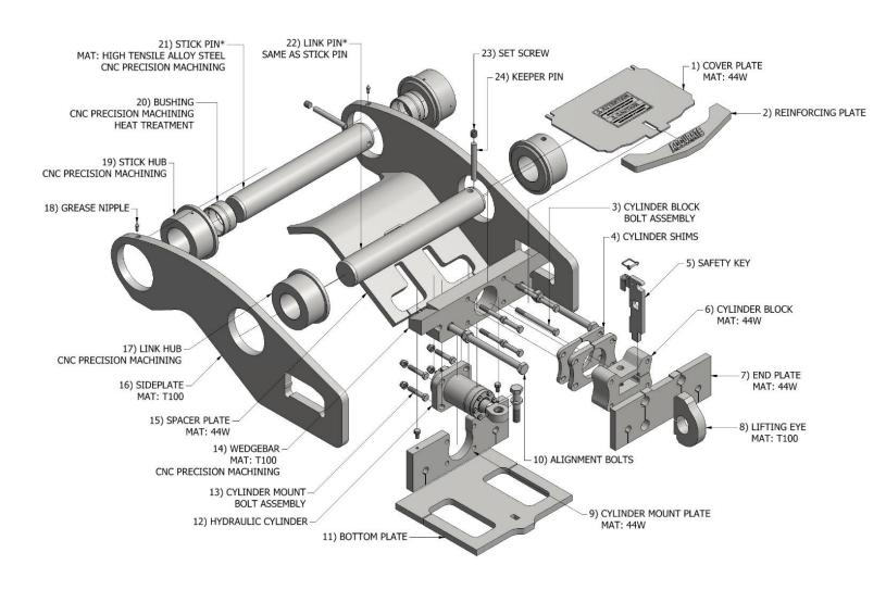
\*Pins are not required for all OEM machine manufacturers.
